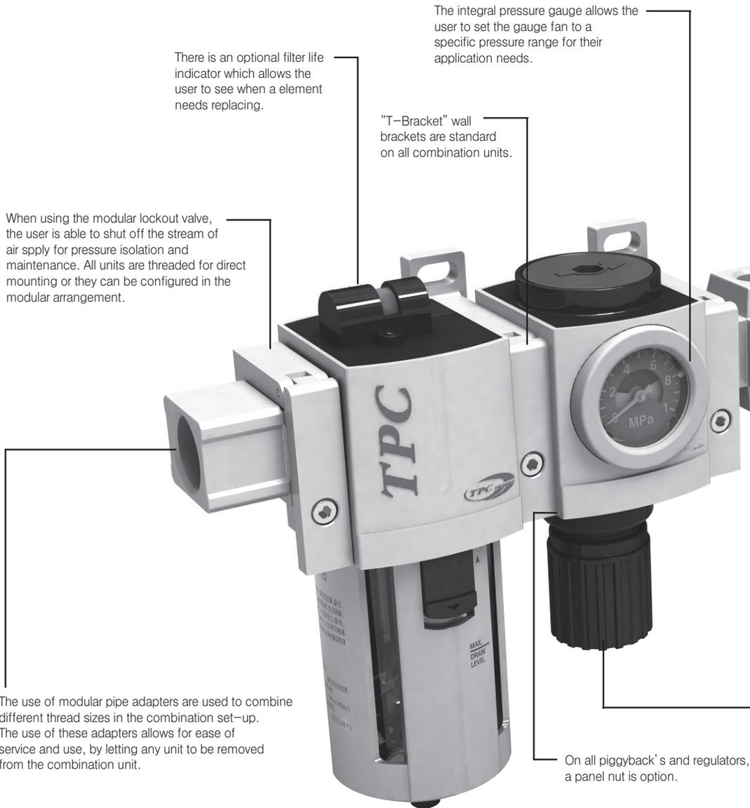
There is an optional filter life indicator which allows the user to see when a element needs replacing.
