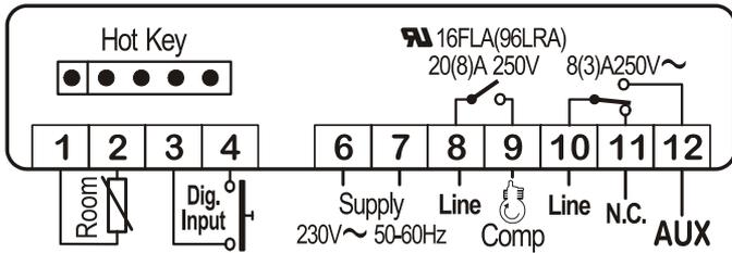
**NOTE:** In model with 110Vac the power supply has to be connected to 6-7 terminal
