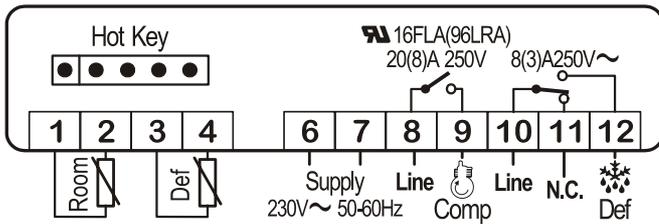
**NOTE:** In model with 110Vac the power supply has to be connected to 6-7 terminal
