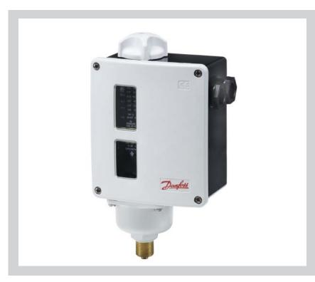
RT Pressure Controls incorporate a pressure controlled, single-pole change over swich where the contact position depends on the pressure in the connection port and the set value.
