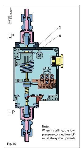
The setting disc (5) becomes accessible when the front cover is removed. The differential pressure is set by turning the disc with a screwdriver while reading the scale (9).
